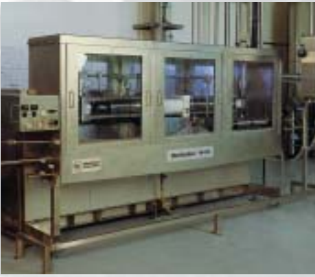
M-610 system used in processing highly abrasive slurry at 9 gallons per minute at 15,000 psi.
